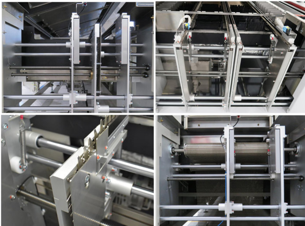
top left: single lane transport, top right: dual lane transport bottom left: lash chain centre board support bottom right: mesh-belt transport 左上：单轨传输；右上：双轨传输 左下：中央支撑；右下：网带传输
